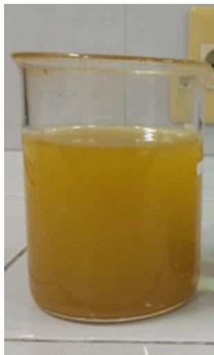
Gambar 4.15 Perendaman Baja ASTM A36 tanpa inhibitor
