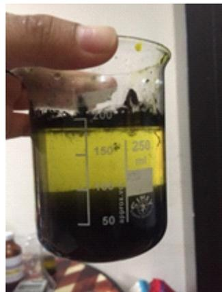
Gambar 2.10 Hasil endapan Graphene Oxide
