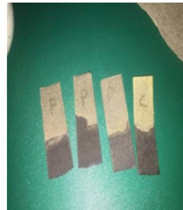
Gambar 2.11 Elektroda Nickel foam GO
