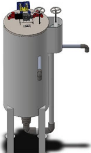
Gambar 6.12 Model Desain *Prototype* Tangki Smart CST Scale Down
