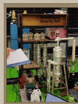
Reaktor Biodiesel *Bubble Column*
