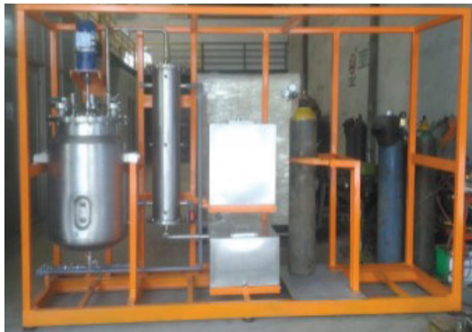
Gambar 3. . Reaktor praperlakuan TKKS pilot plant furfural berkapasitas 100 L
