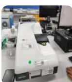
Analisis ukuran partikel fine bubble (Particle Size Analysis dan Particle Image Volumetry)
