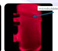
Analisis ukuran partikel fine bubble (Particle Size Analysis dan Particle Image Volumetry)
