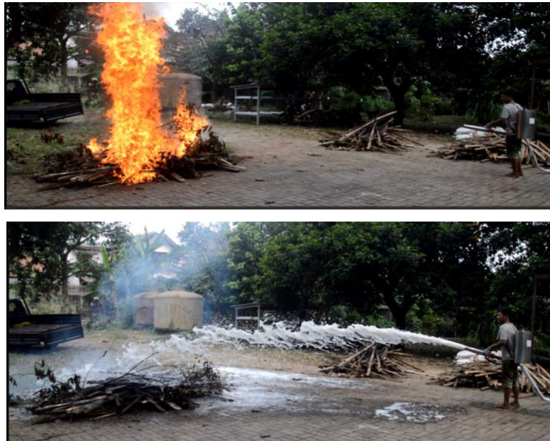
Figure 4. Fire extinguishment trial by using resulted formulas of foaming agent concentrates
