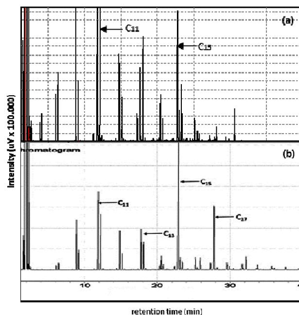
**Figure 3** Chromatograms of biohydrocarbon were resulted in: (a) Mg-Zn(OH)(ME C<sub>12/14</sub>), (b) Mg-Zn(OH)(ME C<sub>12/16</sub>).
