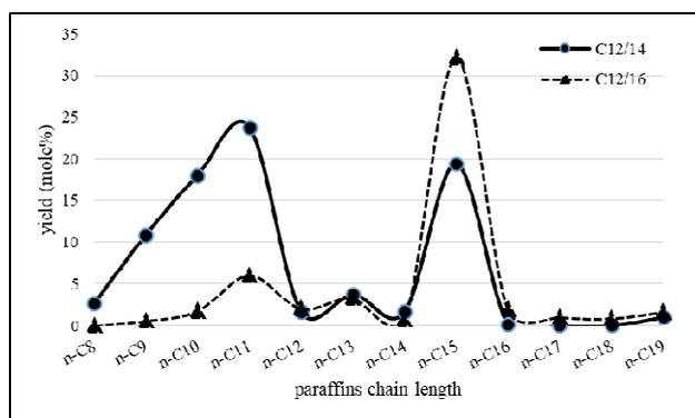
**Figure 4** Relationship between yield and chain length of the n-paraffin fraction.
