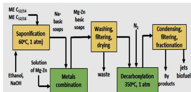
**Figure 2** Flowchart diagram of soap-derived jets biofuel production.
