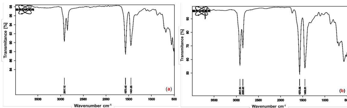
Figure 1 IR spectrum of dried Mg(OH)-stearin basic soaps based on direct method (a) and double decomposition method (b)
