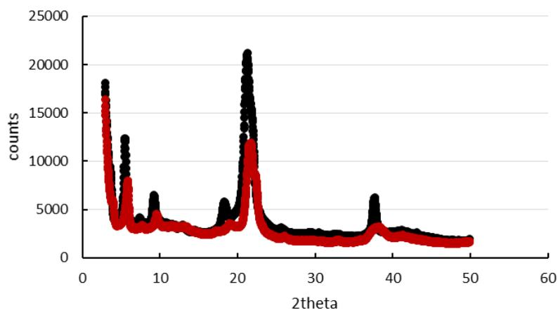
Figure 2 XRD patterns of dried Mg(OH) basic soaps based on direct (●) and double decomposition (●) methods
