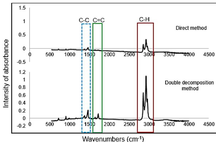
Figure 4 IR spectrum of bio-hydrocarbon fuels generated by decarboxylation of Mg(OH)-stearin basic soaps
