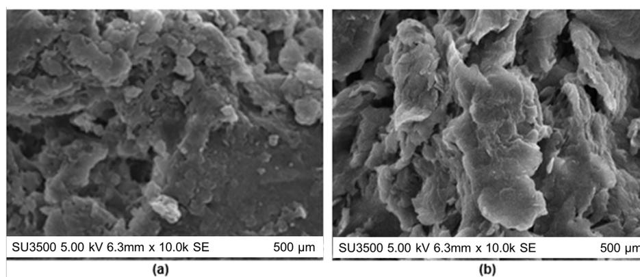
Figure 3 SEM micrograph of Mg(OH)-stearin basic soaps based on direct method (a) and double decomposition method (b)
